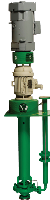
Piggy-back arrangement saves tank space by coupling DC motor with dual- shaft AC motor
