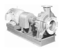
Buffalo Paper Stock Pumps are engineered for high efficiency and designed for ease of service. Back pullout design permits fast removal of the bearing frame, side plate and rotating assembly without disturbing piping. Capacities to 11,000 gpm. Heads to 260 feet. Pressures to 150 psi. Stock handling capacity up to 6%. Bulletin 950.
