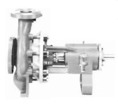
Designed to handle abrasive slurries and solids. **Buffalo Vortex Pumps** feature an adjustable, replaceable vane impeller. One impeller hub size and three vane lengths provide impeller diameters from 7" to 13" at 1/2" increments. Adjustability feature provides modification of pump output and compensation for wear. Capacities to 2000 gpm. Heads to 190 ft. Bulletin 902. Patent Pending.
